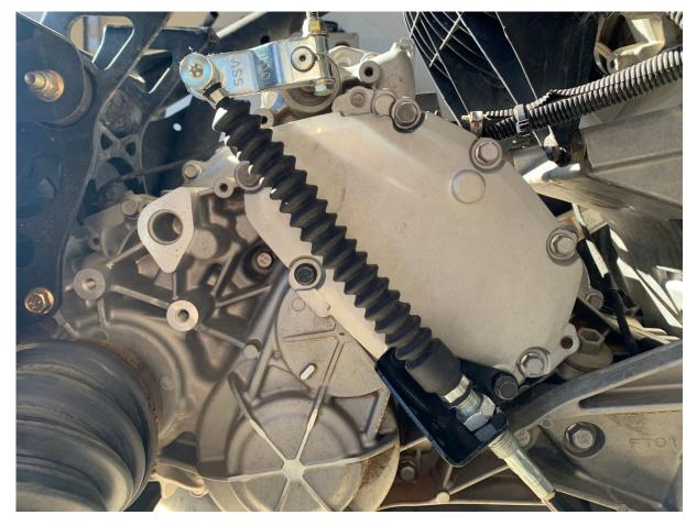
Place the can-am into neutral. Locate the shifting cable and arm.
