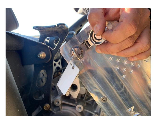
Insert key, turn to lock position, and ensure you can pull key in and out in locked position. If locking mechanism functions correctly, finish installing outside tamper-proof hardware (package C).
