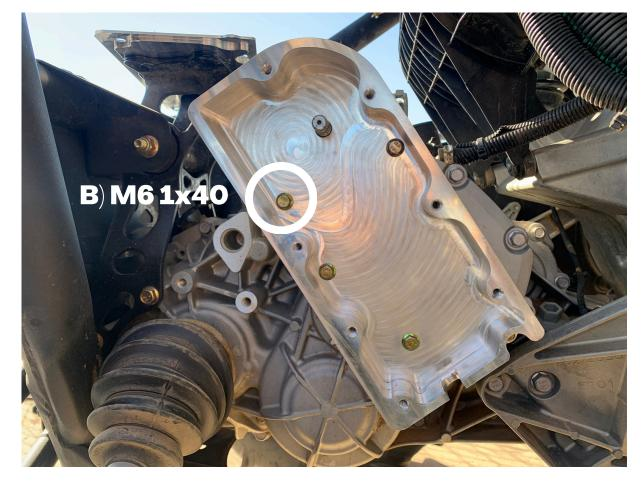
Place the park locker main body over the gear box cover, lining up the shift shaft. Start installing package A & B bolts snug using blue threadlocker. Prior to fully tightening, ensure shift shaft is centered. Torque to 7 ftlbs.
