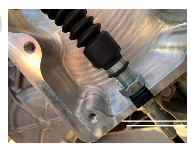
Install the plastic insert with the dove tail facing inward until flush with the edge. Hand tighten cable nuts snug against the edges of the park locker. Shift through each gear and ensure shifter lines up with the detents of the transmission. Adjust cable nuts accordingly.
