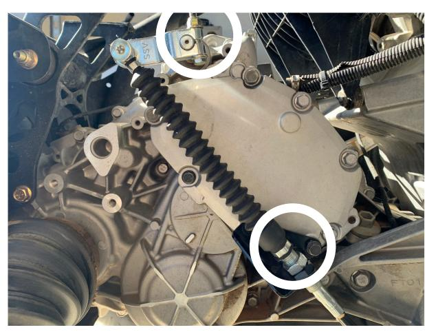
Remove the shifting shaft bolt and nut. Loosen off the cable nuts backing them off at least 1/2". Remove the shifting arm and cable and move out of the way. Remove the two bracket cable bolts and bracket. These will not be reinstalled.
