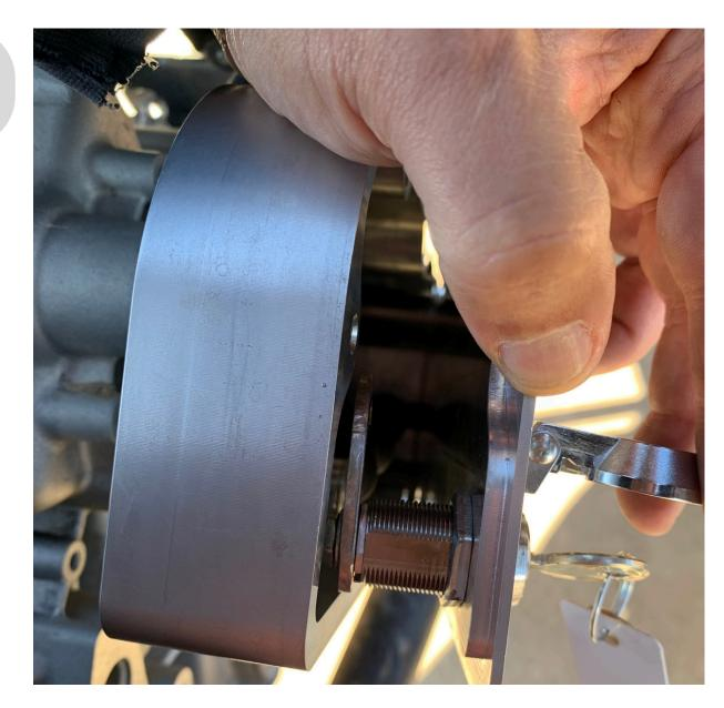
If key is not slightly turned, locking arm may hit inside edge. If lid does not go on easily, try readjusting key turn.
