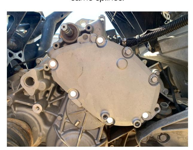
On the gear box cover, remove the following five bolts. (marked here with white dots)
