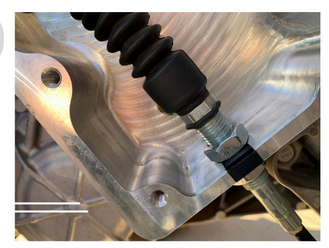
Tighten cable nuts using wrenches pushing towards park locker preventing cable from twisting out. Ensure plastic insert stays near flush with cover edge.
