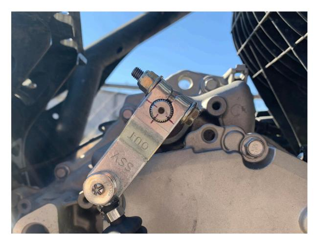
Prior to removing cable, use a permanent marker to mark lines that can be matched up to ensure arm can be relocated back on the same splines.
