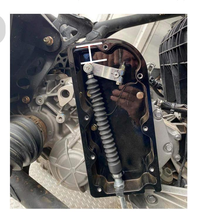
Between the upper inner edge and edge of shifting cable connection (white lines), there should be a 1 inch distance. If the distance between these two points is more or less, rotating the shifting arm on the splines accordingly to achieve 1 inch distance.
