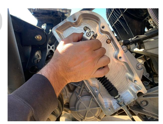
Reinstall shifting arm on shift shaft and insert/tighten bolt. Keep in mind lining up shifting arm with shaft utilizing marker lines from step 2.
