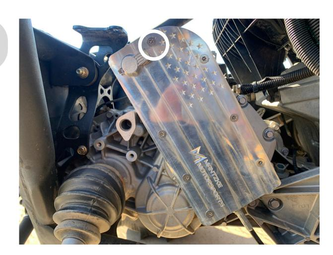
Hand tighten the top tamper-proof bolt (package C). Now, place transmission in park. May have to rock the your vehicle front to back ensuring fully engaged in park.
